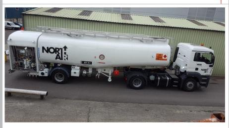
A semi-articulated refueller incorporating a 4x2 chassis and single trailer axle configuration for optimal manoeuvres on the airport ramp. The refuelling unit are mounted on the rear of the trailer tank unit. The refueller is designed and constructed in accordance with the latest European Standards BS EN 12312-5 and JIG 1 Issue 12 requirements where applicable.
